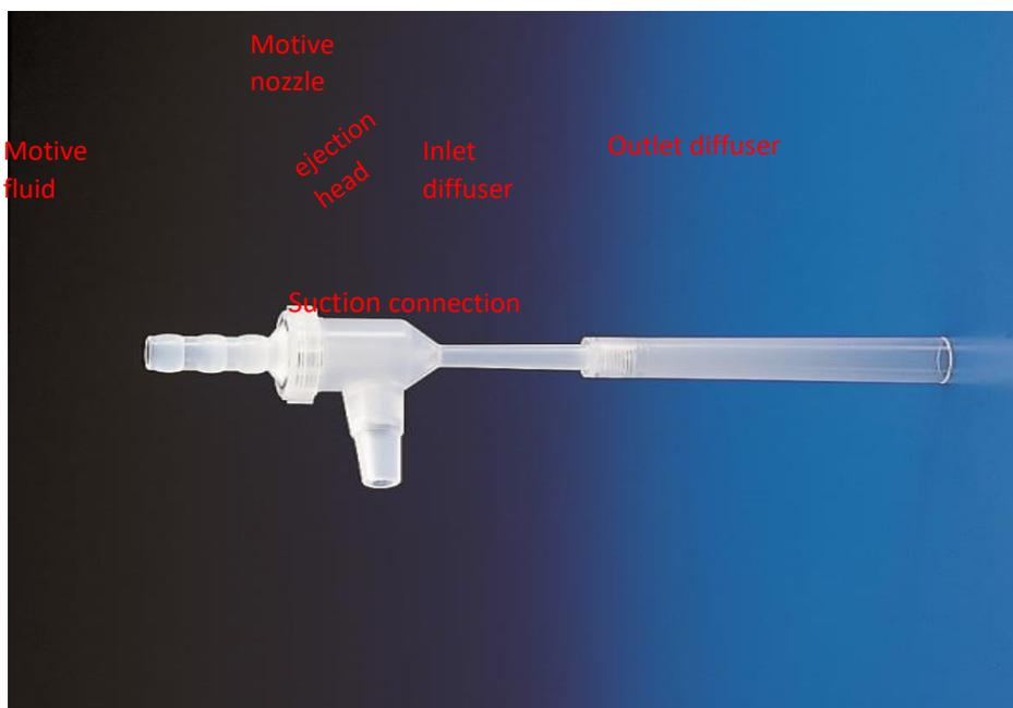
The motive fluid (water) passes through the motive nozzle and the diffuser. The pressure in the motive nozzle decreases and the speed rises.
